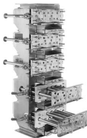
Ten tier 8" x 8" E-Z Clean Drawer Magnet for use in a pharmaceutical application
