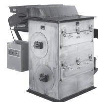
Double Rotating Drum Magnet with Vibratory Feeder
